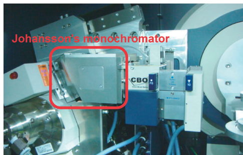
Fig. 2. A unit of K\alpha_1 optical system using a Johansson's Ge(111) curved crystal.
